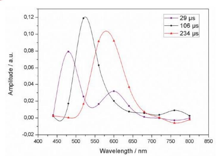
Amplitude-to-wavelength dependence obtained by the ns luminescence technique for Ag<sub>3</sub>K<sub>9</sub>LTA at 77 K in a 1 ms time window.
