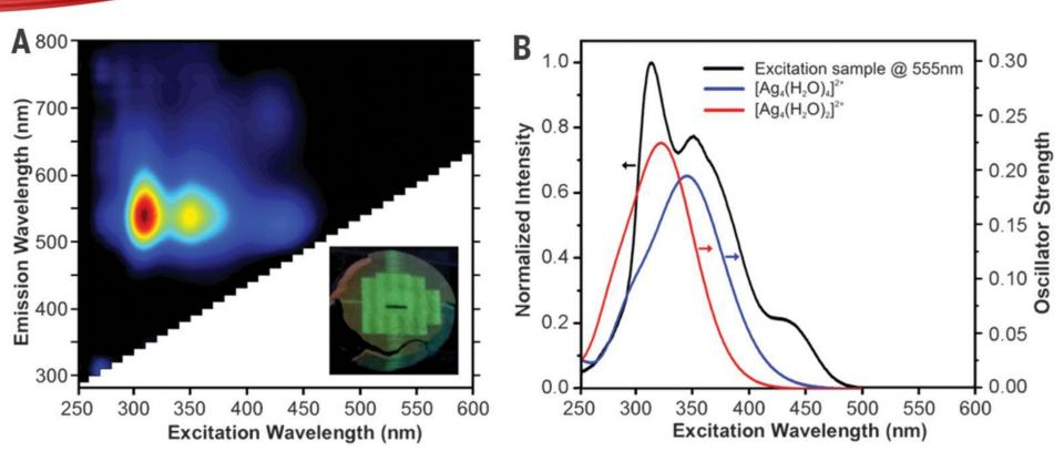
Steady-state excitation-emission of  $Ag_3K_9$ -LTA. (A) 2D excitation-emission plot. (Inset) The picture of an x-ray-irradiated sample under 366 nm illumination. (B) Excitation spectrum  $\lambda_{\text{detection}} = 555$  nm of as-prepared  $Ag_3K_9$ -LTA. Calculated  $^1S_0$  HOMO to  $^1P$  (S = 0; L = 1;  $m_1$  = -1, +1) LUMOs absorption spectra of x = 2 and x = 4  $[Ag_4(H_2O)_x]^{2+}$  isomers showing a good agreement with experiments.
