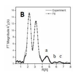
Transmission-detected Ag K-edge  $k_3$ -weighted EXAFS (A) with the corresponding phase corrected FT (B) best fits of heat-treated  $Ag_3K_9$ -LTA zeolite material measured at liquid nitrogen temperature including high-R Ag-Ag contributions up to 6 Å.
