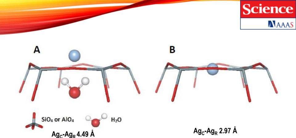
Position of the  $Ag_R$  (blue) at the center of the S6R of the LTA zeolite; (A) outside the sodalite cage when water molecule is present (crystallographic position  $II\alpha$ ) and (B) inside the sodalite cage when no water molecule is present (crystallographic position  $II\beta$ ).
