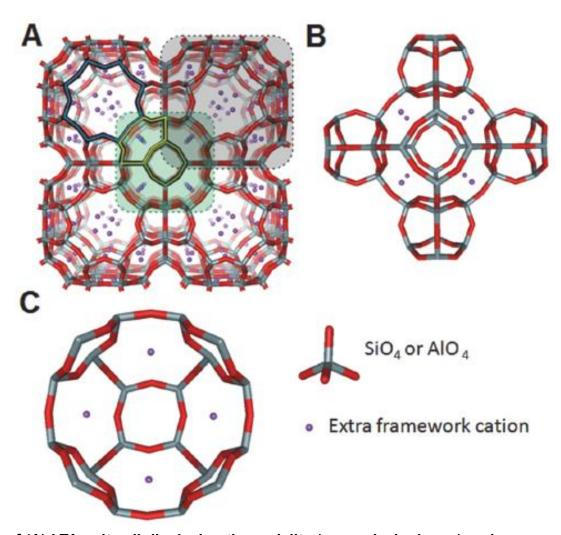
Schematic representation of (A) LTA unit cell displaying the sodalite (green dashed area) and super cage (gray dashed area); the eight ring (8R), single six ring (S6Rs), and double four rings (D4Rs) are highlighted in blue, yellow and green respectively, (B) Isolated sodalite cage with D4R connectors, and (C) Transversal section of a sodalite cage.
