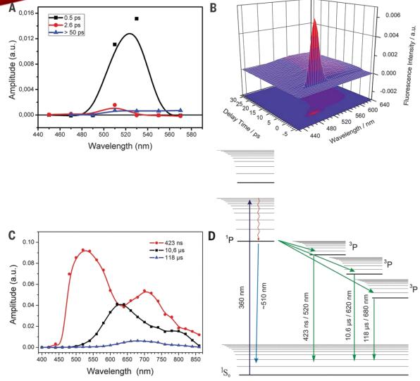
Time-resolved spectroscopy of  $Ag_3K_9$ -LTA. (A and B) AWD 3D time-resolved fluorescence emission spectra in 50-ps time window obtained with (C) femtosecond fluorescence up-conversion, in 1-ms time window through nanosecond luminescence. (D) Schematic illustration of the main electronic states involved as a function of energy (on the vertical axis).
