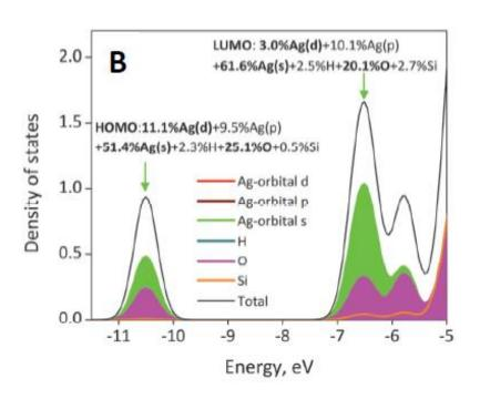
Densities of states of  $[Ag_4(H_2O)_2(Si_{24}H_{24}O_{36})]^{2+}$  (A) and  $[Ag_4(H_2O)_4(Si_{24}H_{24}O_{36})]^{2+}$  (B) (B3LYP/LANL2DZ). The solid line represents the total DOS, the s(Ag) and the oxygen components are shown by the green and the magenta area, respectively.
