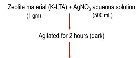
Filtered and washed (several times with milliQ water) the powder sample
