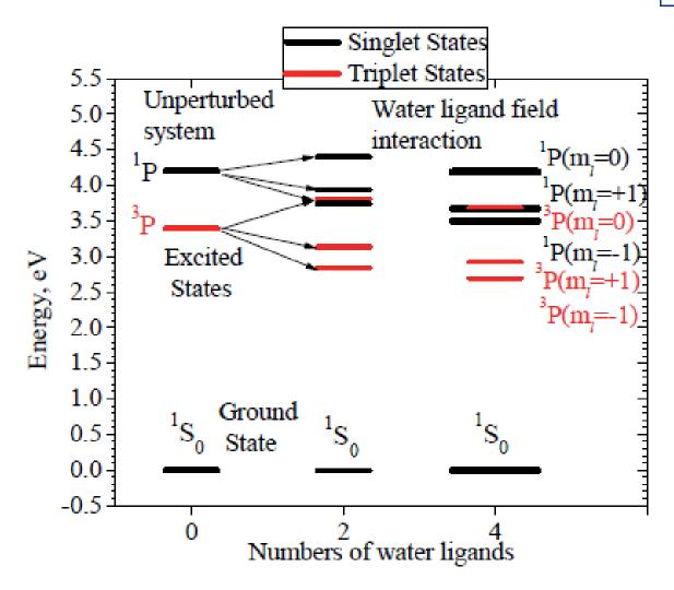
Energy level diagram of the  $[Ag_4(H_2O)_2(Si_{24}H_{24}O_{36})]^{2+}$  and  $[Ag_4(H_2O)_4(Si_{24}H_{24}O_{36})]^{2+}$  clusters calculated using the B3LYP/LANL2DZ functional/basis set.
