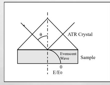
• When angle of incidence ( $\theta$ ) is greater than critical angle ( $\theta_c$ ) results into total internal reflection.
