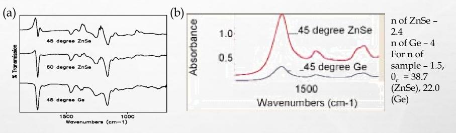
**3.** Efficiency of sample contact – Since evanescent waves decays with distance from crystal surface, hence it is important to have intimate contact of sample with crystal.
