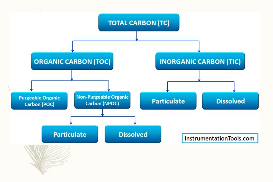
A **total organic carbon analyzer** determines the amount of carbon in a water sample. By acidifying the sample and flushing with nitrogen or helium the sample removes inorganic carbon, leaving only organic carbon sources for measurement. There are two types of analyzers. One uses combustion and the other chemical oxidation. This is used as a water purity test, as the presence of bacteria introduces organic carbon
