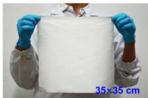
Fabric electrode + P(VDF-TrFE) + PA6
