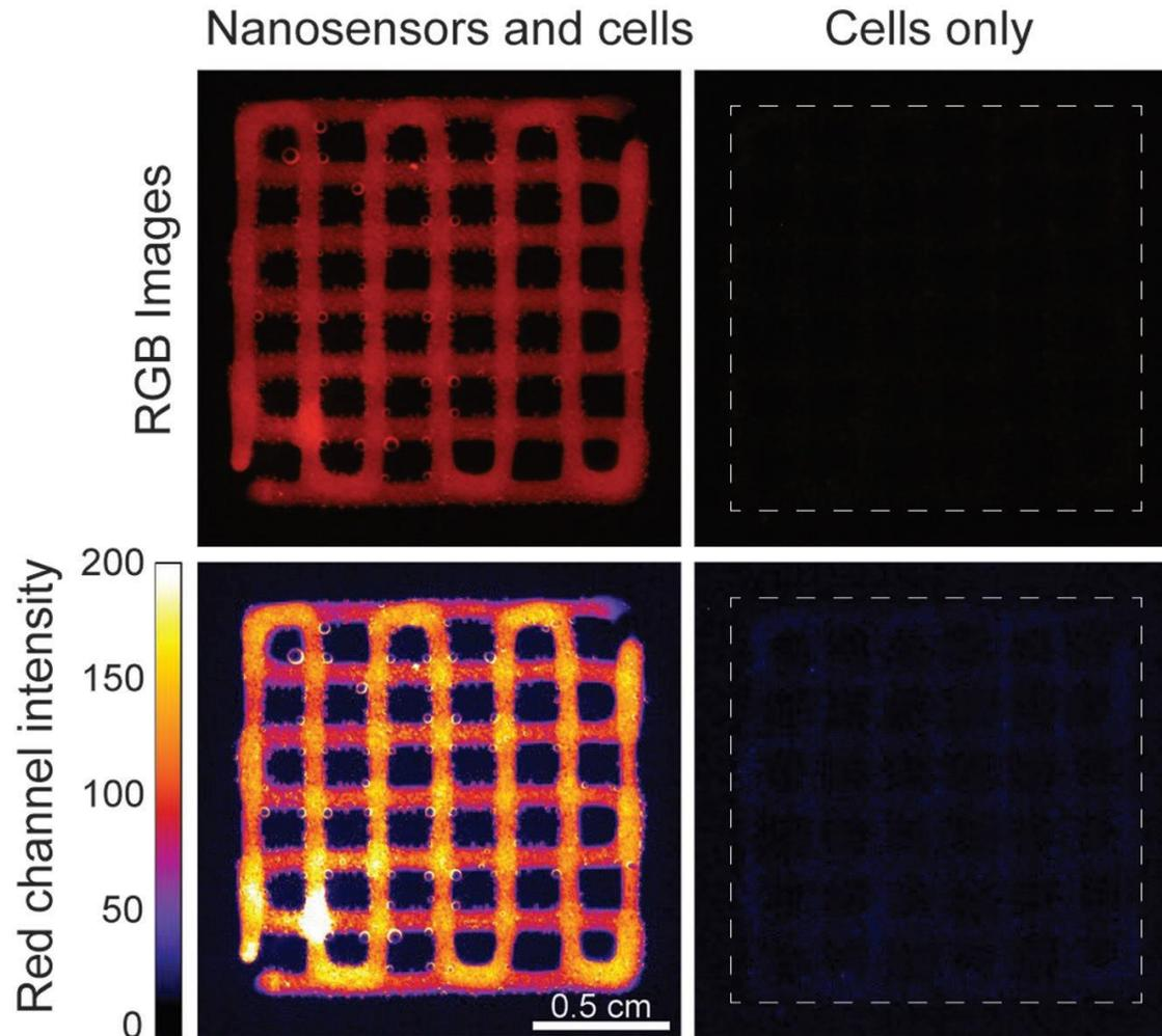
**Figure 4.** Background fluorescence of microalgae (*Chlorella sorokiniana*) as compared to the O<sub>2</sub>-dependent luminescence signal from nanoparticles in the red channel of the recorded RGB image (false color bar). The bioprinted construct was incubated under a photon irradiance of 450  $\mu\text{mol photons m}^{-2} \text{s}^{-1}$ .
