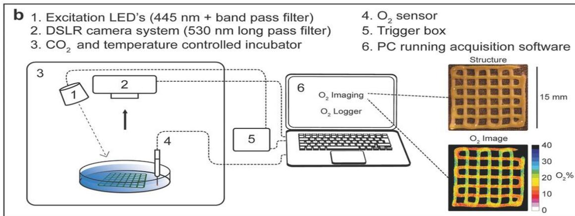
**Figure 1.** A novel approach for 3D bioprinting with bioink functionalized with sensor nanoparticles. a) Living cells and/or nanoparticles in hydrogel blend for extrusion based 3D bioprinting. b) Experimental setup for incubation and imaging of structure and O<sub>2</sub> distribution in 3D-printed hydrogel scaffolds. All components (1–4) besides the LED excitation source trigger box (5) and the PC (6) were placed inside a thermostated incubator with a controlled gas atmosphere.
