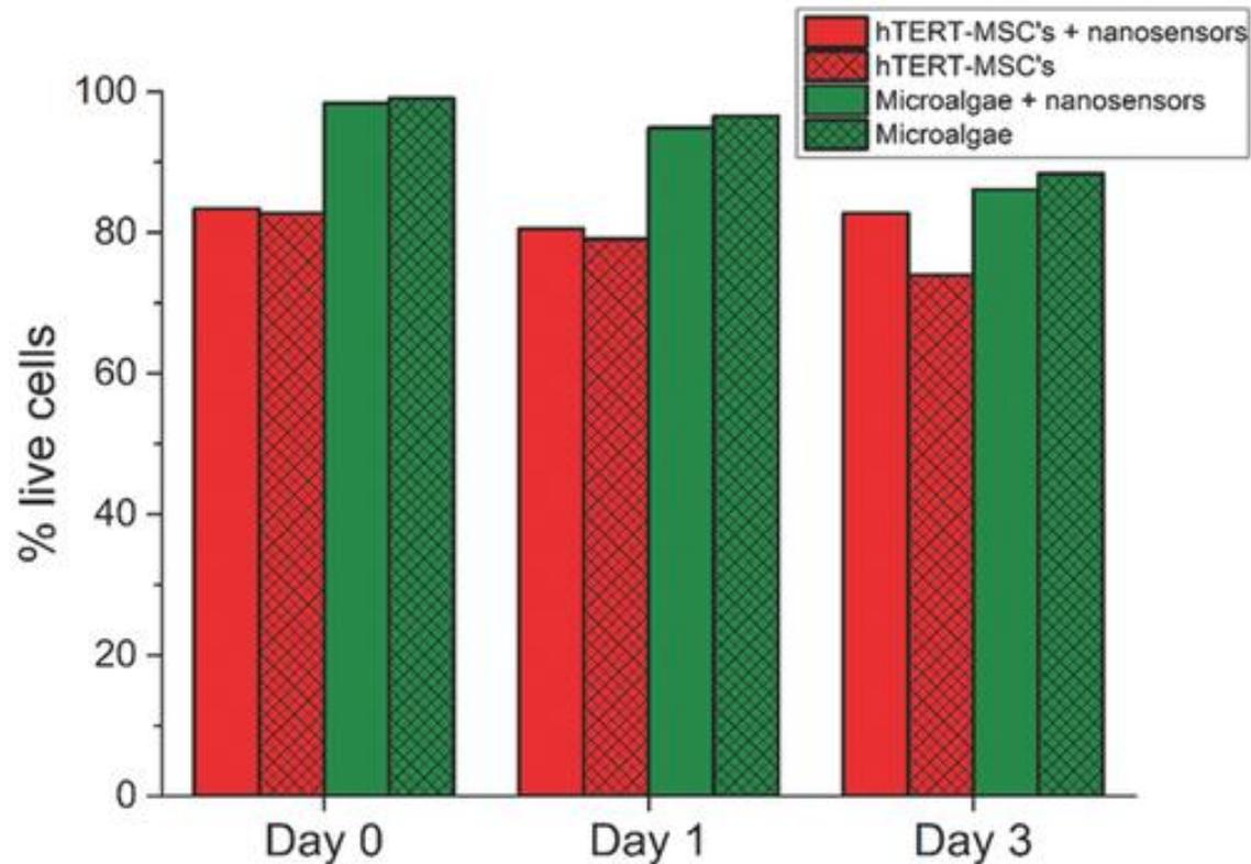
**Figure 2.** Viability of the microalga *Chlorella sorokiniana* and the mammalian cell line hTERT-MSC as a function of incubation time when immobilized in 3D-bioprinted hydrogel scaffolds containing  $O_2$  sensor nanoparticles.
