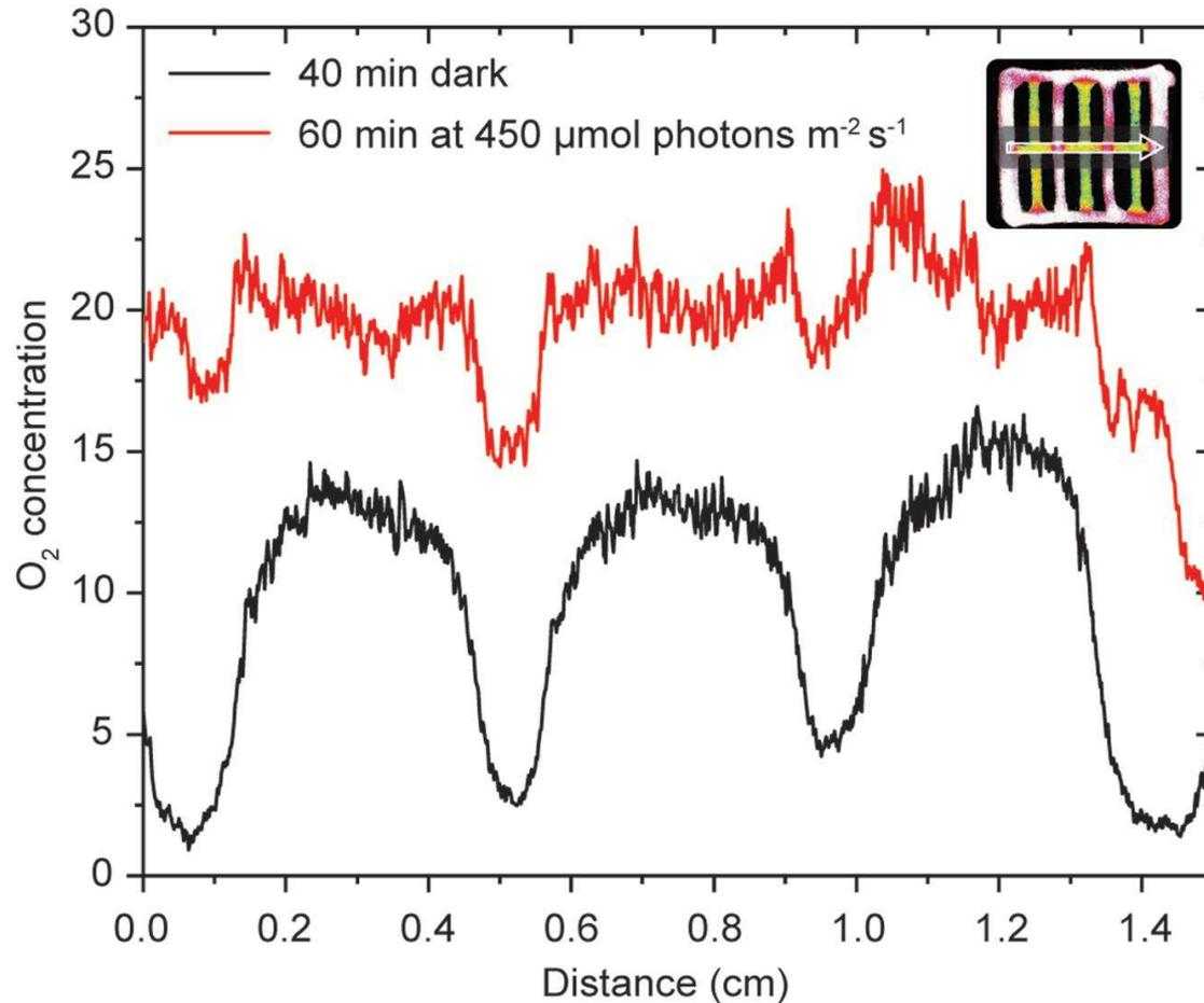
**Figure 7.** The graph shows extracted O<sub>2</sub> concentration profiles across the printed scaffold in a hydrogel strand containing only sensor nanoparticles measured after 60 min light exposure and 40 min of darkness, respectively.
