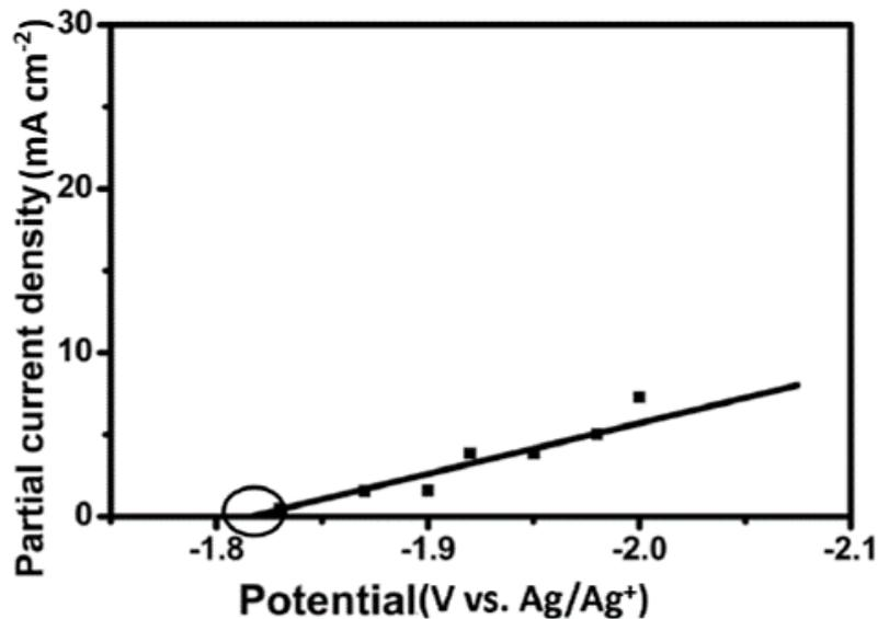
**Fig:** Partial current densities of methanol under different potentials.
