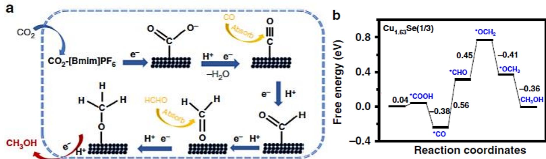
**Fig:** **a** Proposed mechanism on Cu<sub>2-x</sub>Se(y) electrode; **b** free energy diagrams on Cu<sub>1.63</sub>Se(1/3) electrode
