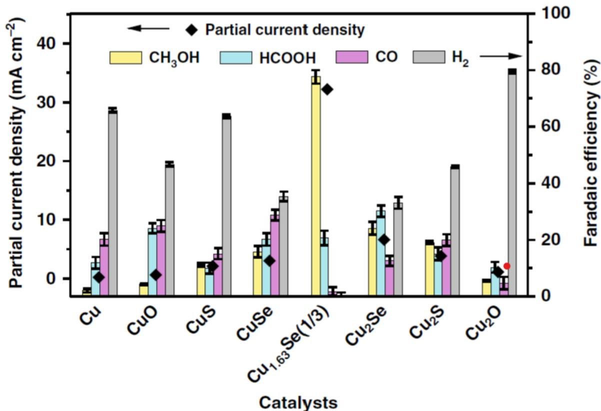
**Fig. 3** Partial current density and FE of methanol over various catalysts at  $-2.1$  V vs. Ag/Ag<sup>+</sup>.
