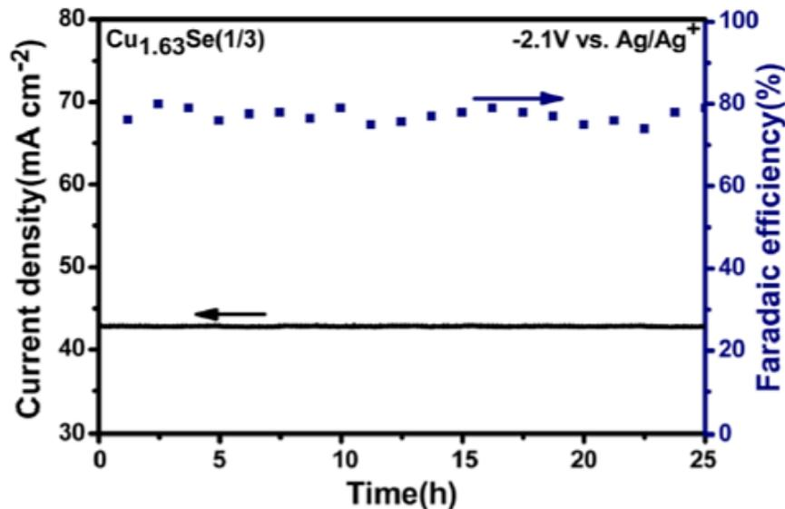
**Fig:** The long-term stability of the  $\text{Cu}_{1.63}\text{Se}(1/3)$  catalyst at the applied potentials of  $-2.1$  V vs.  $\text{Ag}/\text{Ag}^+$
