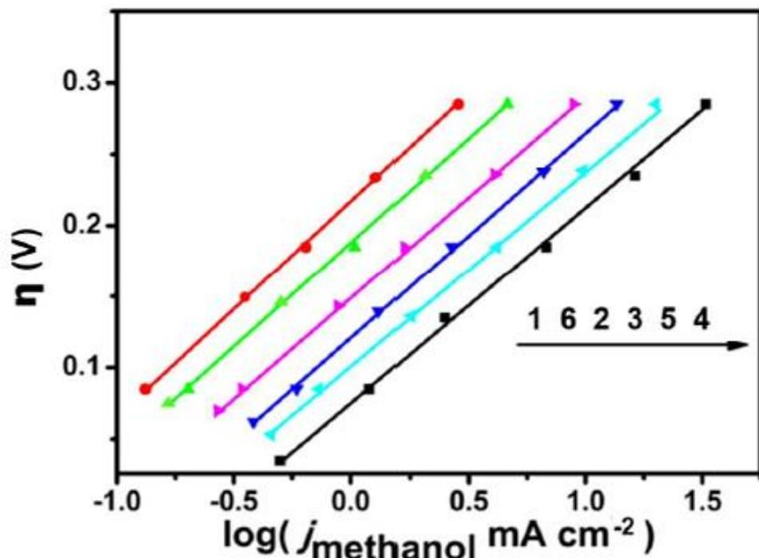
**Fig:** Tafel plot for  $\text{CH}_3\text{OH}$  production over various  $\text{Cu}_{2-x}\text{Se}(y)$  nanocatalysts: **1**  $\text{Cu}_{1.61}\text{Se}(1/0)$ ; **2**  $\text{Cu}_{1.60}\text{Se}(3/1)$ ; **3**  $\text{Cu}_{1.63}\text{Se}(1/1)$ ; **4**  $\text{Cu}_{1.63}\text{Se}(1/3)$ ; **5**  $\text{Cu}_{1.62}\text{Se}(1/5)$  and **6**  $\text{Cu}_{1.64}\text{Se}(0/1)$ .
