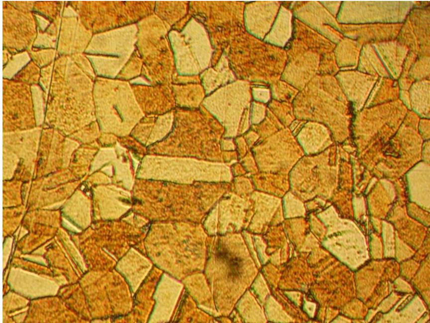
Microstructure of annealed brass.
