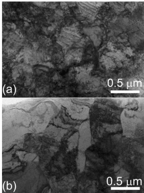
Figure a,b: Typical bright-field TEM images for the  $\text{UFG}_{\text{ECAP}}$  and  $\text{UFG}_{\text{ECAP+D+R}}$  Cu samples, respectively. It is apparent that the grain boundaries in the  $\text{UFG}_{\text{ECAP+D+R}}$  sample are sharper and straighter than in the  $\text{UFG}_{\text{ECAP}}$  sample.
