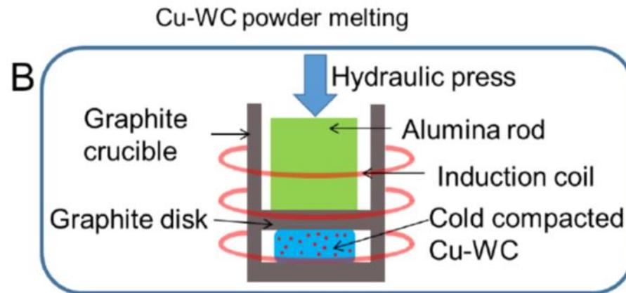
Fabrication of Cu-containing WC nanoparticles. (A) Schematic illustration of the salt-assisted self-incorporation for Cu-WC before casting bulk ingots. (B) Schematic illustration of the powder melting method to cast Cu containing WC nanoparticles.
