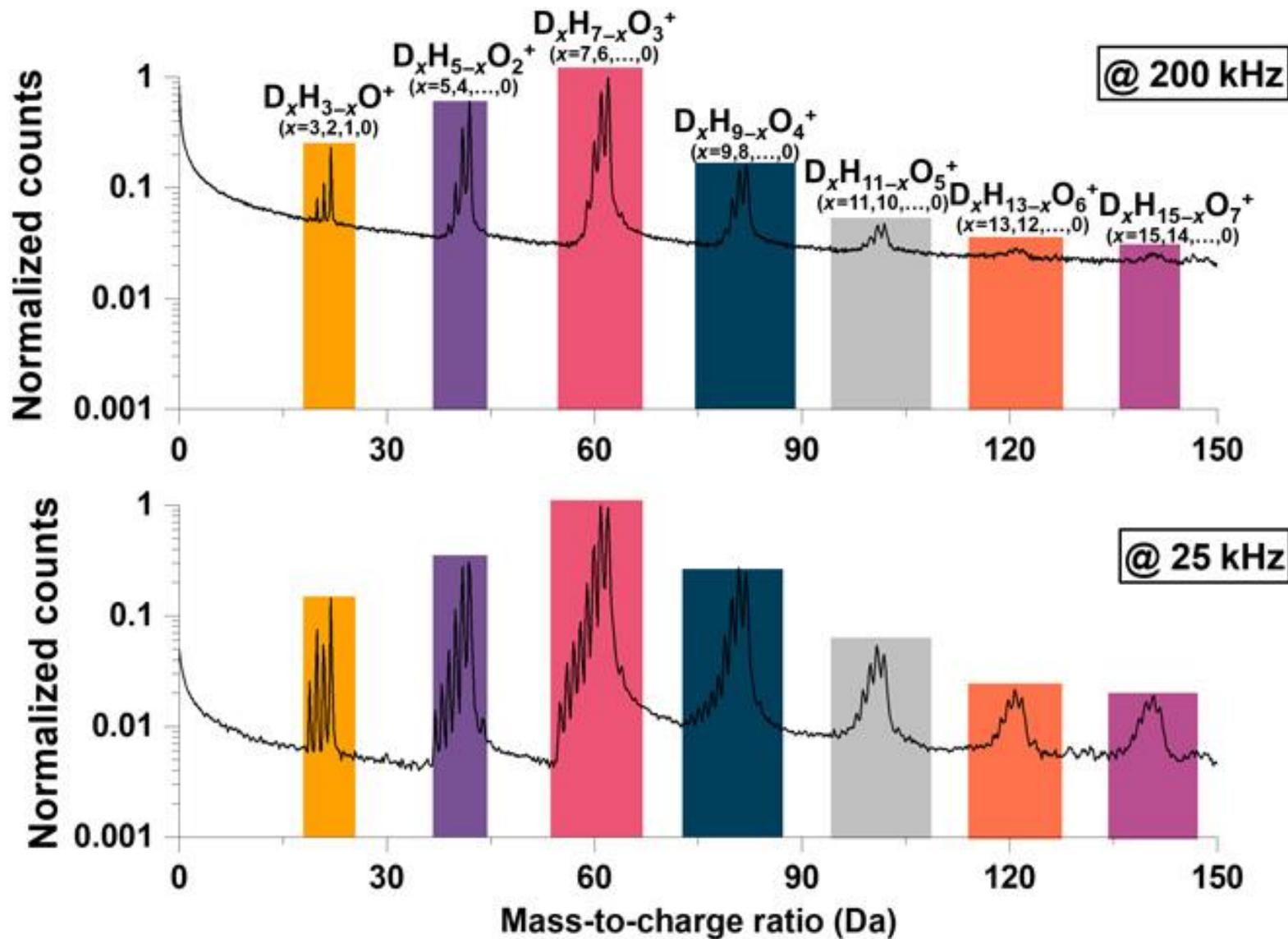
Examples of mass spectra from frozen salt water at different pulse repetition rates. Mass spectra from the NaCl-D<sub>2</sub>O water specimen at 200 and 25 kHz—note the difference in scale on the y axis.
