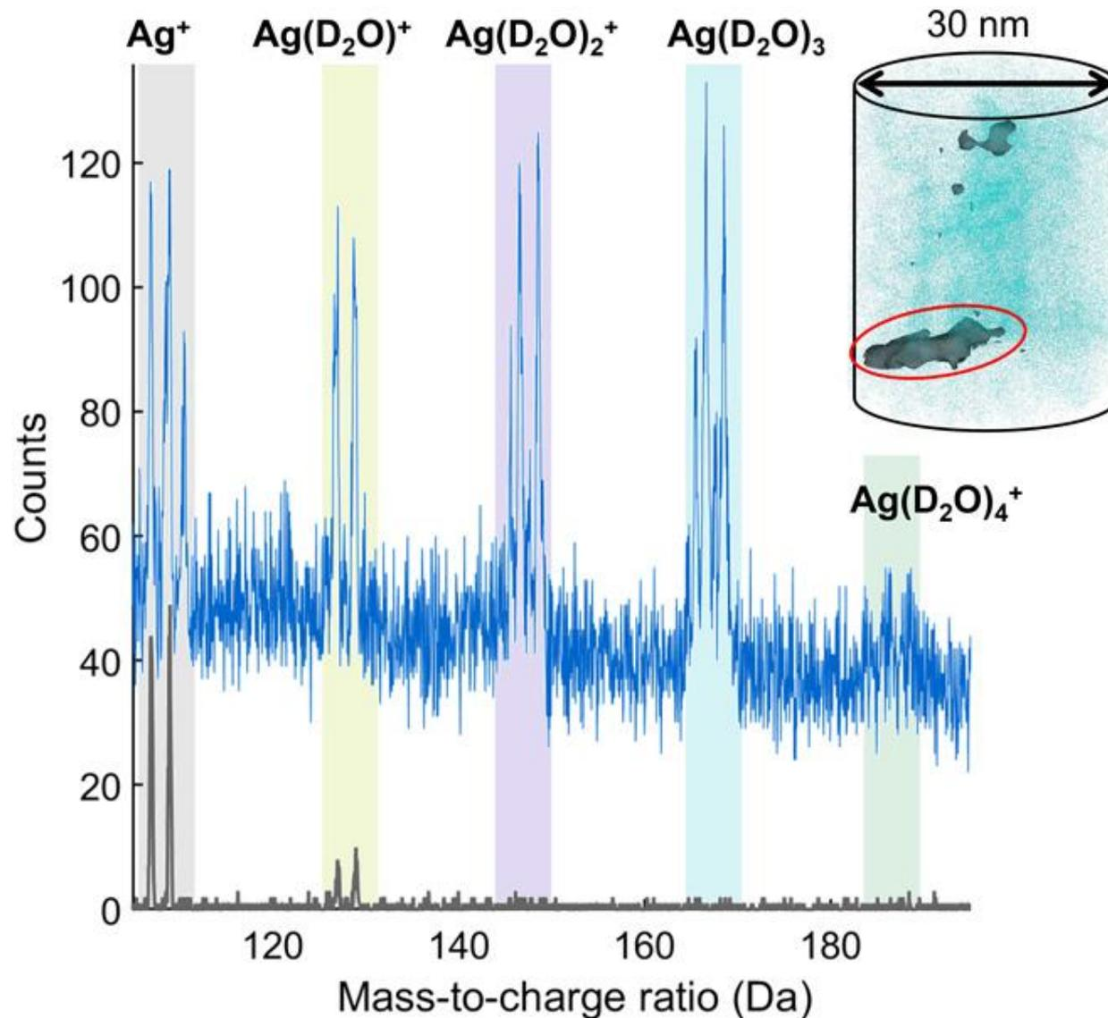
Mass spectra from a floating silver flake and the surrounding ice. Mass spectrum for a 30-nm-diameter and 35-nm-long cylinder, shown in the inset, from within frozen NaCl-containing solution is shown in blue. Inset shows the group of  $\text{Ag}^+$  ions surrounded by ice with an isosurface value of 10 at % for Ag. Mass spectrum from within the flake, marked in red in the inset, is shown in gray.
