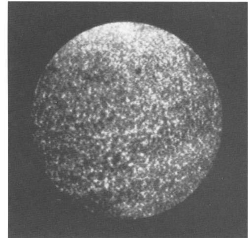
video image of  $\text{H}_2\text{O}^+$  and  $\text{K}^+$  from 1 N KCl in water, frozen on a tungsten tip and field-desorbed from the tip apex. The image shows no order in the liquid indicating that the vitreous state was achieved and maintained during IAP analysis.
