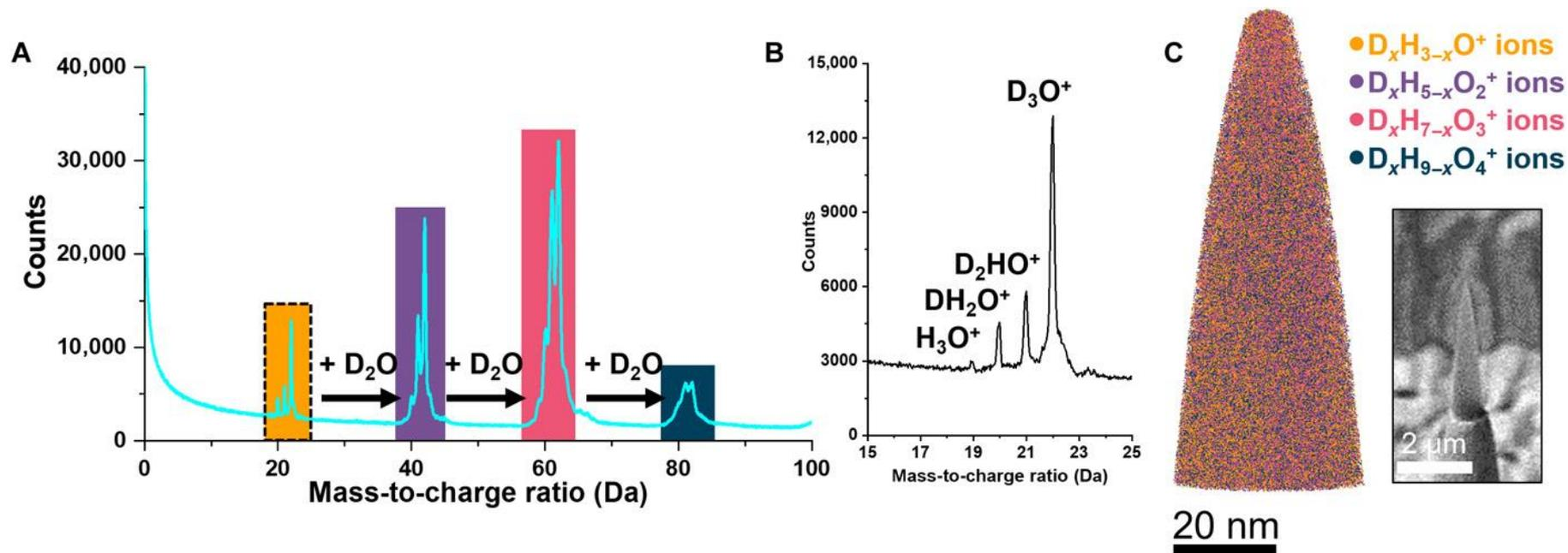
Summary of the atom probe data from a thick layer of ice. **(A)** Mass spectrum of acquired APT dataset of D<sub>2</sub>O ice at 100 pJ, 200 kHz, and a detection rate of 0.5%. **(B)** Sectioned mass spectrum from (A) to illustrate D<sub>x</sub>H<sub>3-x</sub>O complex peaks. **(C)** 3D reconstruction map of D<sub>2</sub>O. Inset capture shows SEM image of the specimen.
