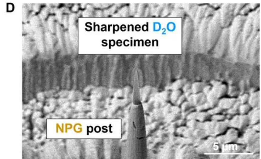
**SEM images of in situ APT specimen preparation of an ice sample on NPG.** (A) The 200- and 75- $\mu\text{m}$  ion beam annular patterns for outer and inner diameters, respectively, were made on the ice/NPG sample. (B) The ice/NPG pillar was milled until the height of the Au post reached  $<50\ \mu\text{m}$  (83). (C) Ice layer was gradually sharpened along with NPG until the layer reached  $<5\ \mu\text{m}$  in height. (D) Final APT specimen of ice on NPG.
