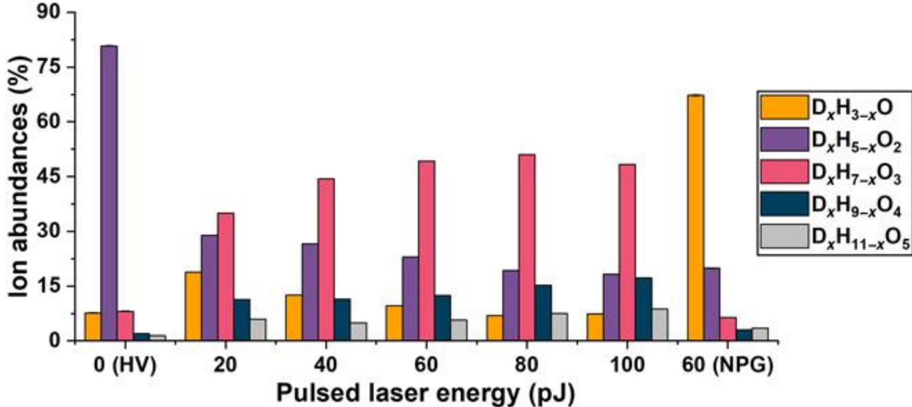
Relative molecular ion abundances as a function of the laser pulse energy and in high-voltage pulsing mode. Relative amount of different cluster ions observed in the analysis of  $D_2O$  ice at pulsing energies ranging from 20 to 100 pJ. Pulsing fraction for the HV measurement was 15%.
