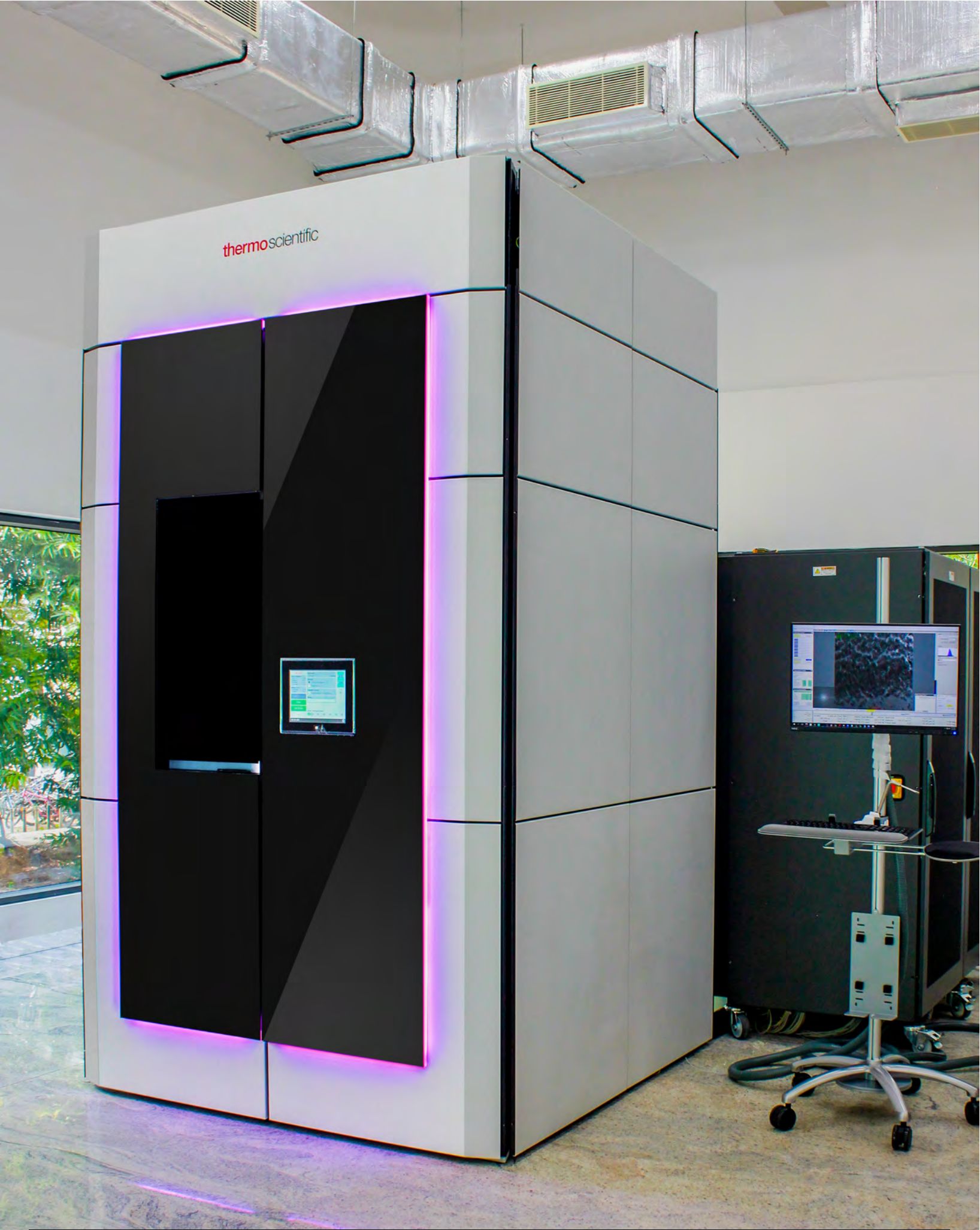
Our cryo-EM facility houses a Titan Krios G4, a 300 keV top-of-the-line microscope equipped with Falcon 4 direct electron detector.
