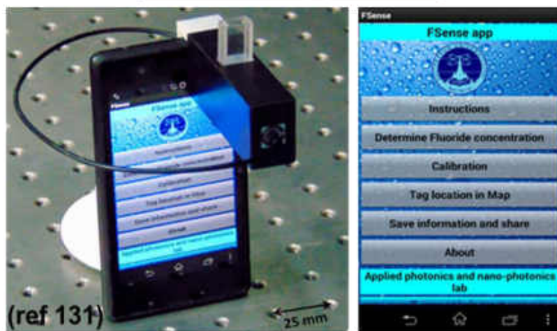
Cost-effective sensor accessory for point-of-use applications
