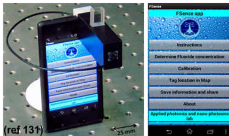
Cost-effective sensor accessory for point-of-use applications
