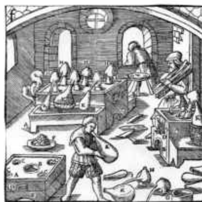
A—Furnace. B—In which wood. C—Alchemist. D—Mouth of the furnace. E—Chamber where wood is. F—Alchemist's crucible. G—Alchemist. H—Chamber. I—Alchemist. K—Other apparatus. L—Alchemist in which wood is placed and it should be heated.
